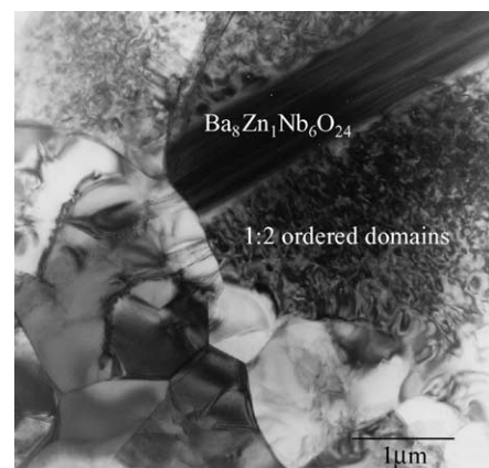
Fig. 5. TEM image of BCZN ceramics.
